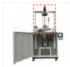
Pneumatic cylinder for lifting cover
