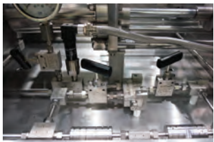
Easy to remove clogging by back-flushing
