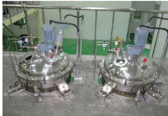
超临界水热合成设备 Supercritical Hydrothermal Synthesis system
