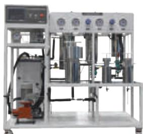
超临界萃取系统 Supercritical carbon dioxide extraction system
