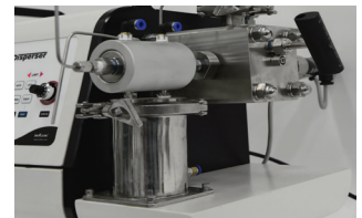
Cooling tank after process
